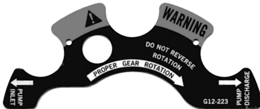
TYPICAL DIRECTION OF ROTATION TAG FOUND ON RV STYLE RELIEF VALVES
